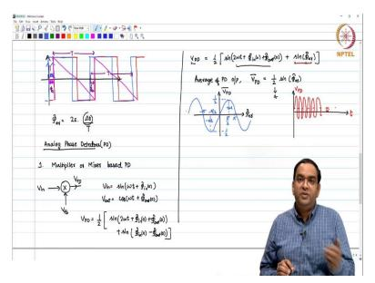
So, in this case, we know that this is a mixer which multiplies the two signals. You are going to use this phase error detector only when you have sinusoidal signals. So, these are  $V_{in}$  and  $V_{fb}$ . I call the output of the phase error detector as  $V_{PD}$ . I am not calling this as phase error right now. This is the output of the phase error detector. So, this is  $V_{PD}$ . Given that,
