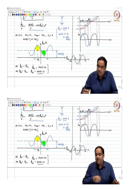
If such is the case which you see here when the PLL does not lock, this is the same thing which I did not tell previously, but I showed you that the waveform just keeps on doing something like this. And you know that this error voltage is passed as the control voltage. And when it is passed as the control voltage ( $V_c$ ), even the control voltage ( $V_c$ ) will do the same thing and the PLL is never going to lock.
