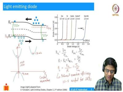
So, what is the light emitting diode? Well, a light emitting diode is very similar to a pn junction. So, this is a band diagram of a pn junction in forward bias you have seen it many times so, far in this course. So, essentially here we are applying a forward bias so, there is a difference in the quasi Fermi levels. So, this will be your  $E_{Fn}$  and this will be  $E_{Fp}$ . So, the splitting of Fermi level happens because we are applying voltage.
