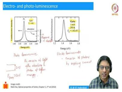
Luminescence is basically emission of a photon. We can have photo luminescence photo luminescence, which is essential you know shine a photon. Like for example, I take a semiconductor, which has a bandgap of 2 eV, I shine light, which has an energy of 2.5. eV, and then I will make it emitted 2 eV. If I have a bandgap, for example, the bandgap, in this case, 2 eV I can shine any photon of higher energy.
