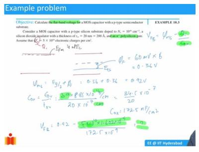
Wherein we want to find out what is the flat band voltage for a MOS capacitor which is having you know p-type substrate, let us say. So, I will not solve this problem. I will quickly tell you how to do this. So, you are asked to calculate the flat band voltage.
