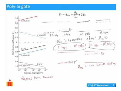
So, how does polysilicon work? So, what we will do in this case is let us say you have the same you know p-type substrate. There is an  $E_F$ . What if I use a p plus doping for my gate p plus poly in p type? Or, I could use n plus poly I mean n plus means  $E_F$  is close to  $E_C$ . p plus means  $E_F$  is close to  $E_V$ . There is a sorry I will take an n type here. n type and then this is n plus poly.
