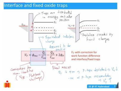
So, this is one form of non-ideality. There is another form of non-ideality that we would like to study which is basically the formation of traps in the oxide. So, in the assumptions for an ideal MOS capacitor we said that there are no traps in the oxide and the interface between silicon and silicon dioxide is perfect. You know there are no traps there as well. But again this is not a very accurate assumption.
