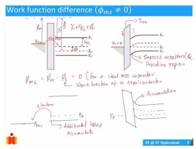
So, to start with, if you remember we have assumed that the metal and semiconductor Fermi levels are at the same point. That means the work functions are same. In other words, now, we define  $\Phi_{ms}$  as a quantity.. So,  $\Phi_{ms}$  is a quantity which is the difference of work function in the metal and the semiconductor.
