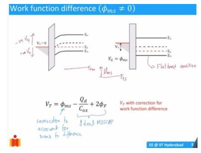
Like for example, I just we have read on here this is the depleted state. And we have said that whenever you apply positive gate voltage to the metal, it will move down move down positive  $V_G$ . If I apply negative  $V_G$ , it moves up, the Fermi level of the metal moves up. So, now, what we can do is apply a negative voltage such that you pull the metal Fermi level up. So, that will force the bands to become again it come into the flat band condition.
