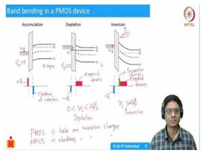
So far, we have discussed only the NMOS device. So, we have taken a p type substrate, but in a PMOS device, we have to take an n type substrate. You take an n type substrate and then
