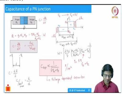
And it turns out that there is definite capacitance in a diode and at least in one of the forms, it is relatively simple for us to analyze. So, look at. Think about this. So, you have a PN junction with an applied voltage. And for now, we will consider the reverse bias. We will not look into forward bias; only the reverse bias. So, what happens in the reverse bias? What is often a capacitance?
