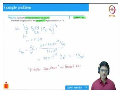
Well, this is again a problem from the textbook 7.5. You can go back and verify the solution as well. And you are asked to calculate the junction capacitance for a PN junction assuming, all the parameters are not given, but they are all from another example. So, if you are asked to calculate the junction capacitors, first thing you will do is simply the width of the depletion region:
