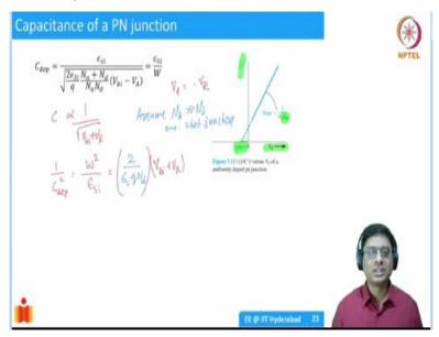
One of the important points is. So, if I look at capacitance, as I said, just a moment back, it is 1 over root of voltage. If I write VA = -Vr. And applying reverse bias that is all I want to explicitly make it clear.
