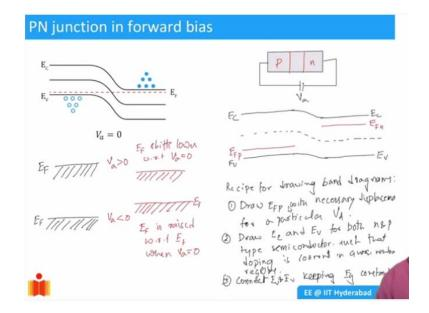
So, we want to understand this in terms of the energy band diagrams. So, we have already seen the equilibrium energy band diagram at no applied voltage. Now, what happens to the energy band diagram when you apply a voltage? So, what we are essentially doing is we are taking a PN junction and then we are biasing it. So, when the positive voltage positive terminal is connected to the P type semiconductor, what happens?
