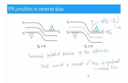
So, the same analysis we can do for the reverse bias as well. So, in the case of reverse bias, if you carefully work out this, you see that the Fermi level has now Fermi level of the P type semiconductor has moved slightly up. This is  $q(V_{bi}-V_a)$ , but now  $V_a$  is negative. So, the whole thing is basically slightly shifted up the barrier. So, this difference in Fermi level is simply  $qV_a$ .
