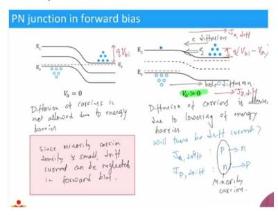
Now, we can quickly understand what happens in the forward bias. The same thing in a slightly better way it is definitely much better than my diagram but essentially same thing with additional electrons and holes shown here. This is for voltage which is positive. Now, what happens when you have such a scenario? When you had no applied bias, we said that there was no diffusion possible.
