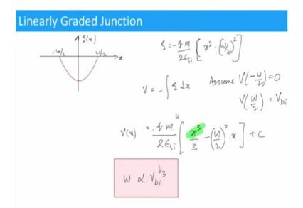
So, what happens to the potential built-in potential? It is of the form  $V(x) = \frac{qm}{2\epsilon_{Si}} \left[\frac{x^3}{3} - \left(\frac{W}{2}\right)^2 x\right] + C$  with depletion width,  $W \propto V_{bi}^{\frac{1}{3}}$ .
