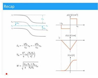
So, in the last lecture, we discussed the PN junction in some depth. We derived expressions for the electric field and the peak electric field at the center of the depletion region. And then we also derived expressions for the built-in potential and the width of the depletion region. So, I mentioned that the width of the depletion region plays a very important role because a lot of the junction physics is essentially that. So, today we will try to move forward.
