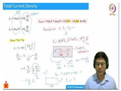
Drift current also is going to be significant. We have to take both into account. So, when you would have diffusion. So far, we have seen that doping was very uniform, the E<sub>C</sub> was constant, so the density was constant all the time. Whenever you have density constant,  $\frac{dy}{dx}$  is going to be 0 so, diffusion is not going to be there.
