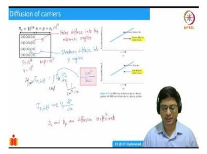
So, now I would like to introduce another type of carrier conduction, which you call as diffusion. We have seen drift which is essentially a result of electric fields, which are applied to the semiconductor. And diffusion is basically a result of concentration gradients. For example, think of a semiconductor, which is a hypothetical case here; we are having a semiconductor with some carriers.
