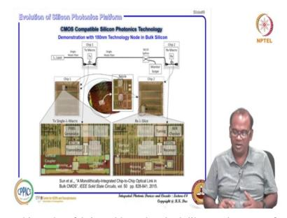
So, this is the same thing when fabricated how they look like you have a wafer this is your wafer and if you see the wafer 1 reticle that is actually is very well known in VLSR technology when you will do photolithography all CMOS technology. So that particular window can be exposed at a time that is actually a reticle that particular reticle by reticle you can just export and process different type of exposure for photolithicol purpose.
