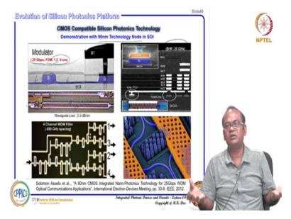
So, later on in 2012 Intel's research actually sold that actual they fabricated using their CMOS technology which the 90 nanometer technology node this modulator they fabricated you see this is the waveguide and this is the slab region we are actually put make doping p type or n type doping so that carrier inside the waveguide region you can control so that refractive index you can actually control and this is the signal with via metal M1 metal you are giving here.
