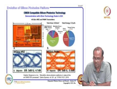
And then the demonstration with 40 nanometer technology note in SOI. So that is happened also with IBM technology IBM actually demonstrated 45 nanometer technology you see parko integration of photonics and electronics you see that is a digital phase locked loop driver serializer you are using all these things serializer this is optical interconnect whenever you are seeing that I will discuss that how they can be serialized in course of time.
