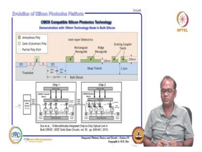
And then as I said that that co integration I showed the figure earlier that photonics and electronics can be co-integrated in using bulk CMOS bulk silicon with CMOS technology and it was also another demonstration from IBM 180 nanometer technology they have used to co integrate this per example transmitter right I think they have used too many more ring resonator it is a lambda 1, lambda 2, lambda 3 you can go for 100s of channels 100 ring resonator.
