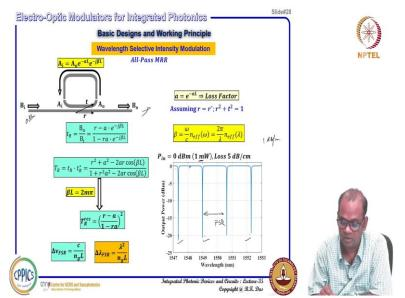
Now see as you if I consider the input here you are just considering 0 dBm or 1 milliwatt power - 0 dBm is equivalent to 1 milliwatt just 1 milliwatt you take the log scale so then you get 0 so because milliwatt we consider this 0 dBm I think all of you know that how to do that and loss again we consider the waveguide loss is about 5 dB per centimeter nowadays waveguide loss can be reduced to 1 dB per centimeter as well.
