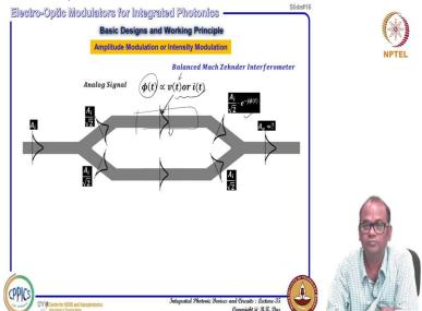
So, now you see suppose in a balanced Mach-Zehnder interferometer you have a phase you are adding here to this mode in the upper arm which is time dependent and this phase can be changed in terms of voltage time dependent voltage or time dependent current that is eventually your can be your analog signal or digital signal as a function of time voltage can be fluctuating depending on the data current can be fluctuating.
