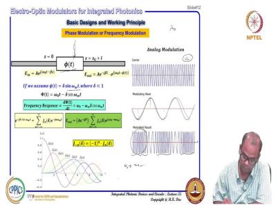
Now you see if you try to see analog modulation that means this phi t can be a function of time with sudden modulation like this, this type of analog modulation not like that phi t is a step function just a 0 or some values instead of that as a function of time it is changing your data can be your incoming data whatever data is coming that can be also certain kinds of any value it can take.
