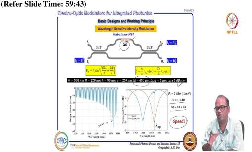
So, I see that same thing we discussed about your in case of here so it is almost similar type of thing insertion losses about 1.2. Similar type of waveguide structure will consider same type of delta 1 we consider in the unbalanced arm difference in arm length and micro ring resonator also we consider the ring resonator length 450 micrometer so FSR is almost similar. So this FSR we consider about 1.6 nanometer or about 200 gigahertz in frequency domain.
