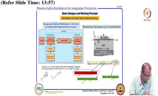
Now you see you can actually modulate the polarization, polarization you can have suppose you have a x component and a y component. So, what you could do? You can actually somehow you can change the polarization components that means E x fraction if you can just modify to higher level and E y fraction can be reduced to the lower level for a given power or amplitude of the electromagnetic wave.
