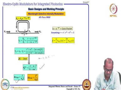
So, now you see we know that at the resonance condition transmission will be this one where beta l = 2 pi times integer m = 1, 2, 3, 4 so on and we know that also for a ring resonator this delta FSR frequent pre spectral range for the ring resonator c / n g L and in terms of lambda, lambda square by n g L that we know that earlier.
