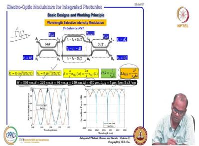
So, we have just simulated for a certain waveguide structure where waveguide with you know this type of waveguide to consider in silicon this is the W and this is H and this is a small h. So if you are considering W = 500 nanometer device layer thickness equal to 220 nanometer h = 90 nanometer and gap g this g means when you are designing a directional coupler that gap is we are considering wave guide to wave guide separation is 250 nanometer.
