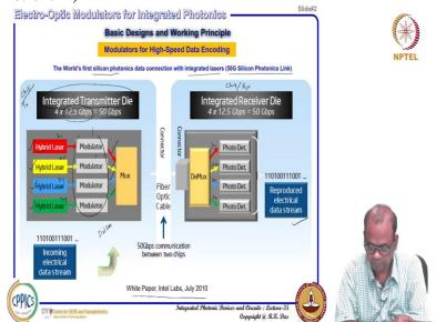
So, let us see how modulators play a major role in high speed data encoding. So, here I have tried to given an example borrowing a photograph the scheme from Intel Labs white paper this was depicted in 2010. So, when they actually demonstrated the world's first silicon photonics data connection with integrated lasers, 50 gigabit per second silicon photonics link. So, before that actually high speed modulators being used for long haul fiber optic communication.
