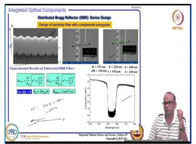
Now, you see such a device actually we have developed we have understood the coupled mode theory now, that this is possible. Now, I have shown that some device we fabricated in our lab in IIT Madras. I see this is the how waveguide a scanning electron microscopic image it is shown here. And the DBR Design you define in a periodic perturbation and fabricate then finally we end up with this type of structure both side details perturbation is there.
