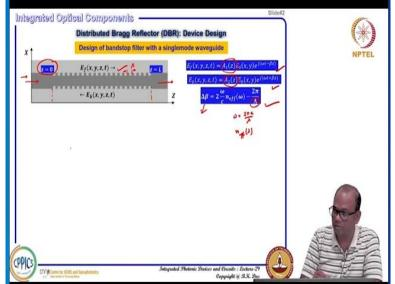
So now, let us again recap the DBR structure it is basically top view of representative silicon on insulator waveguide structure. So, this is your waveguide you can consider this is your single mode waveguide, this is also single mode waveguide output and input also single mode waveguide but in between from z = 0. So, from here to here z = L this is z direction, there is a periodic perturbation.
