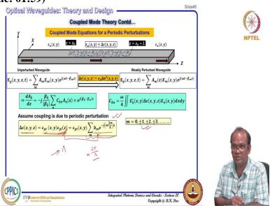
So, let us move on, so here we start with a coupled mode equations for general periodic perturbations. Here we have shown some perturbation we have shown that perturbation when it is actually uniform waveguide which is defined by dielectric constant means under epsilon a, x, y that means epsilon a, x, y earlier we have defined something like this epsilon 0 n square a waveguide cross section refractive index profile square.
