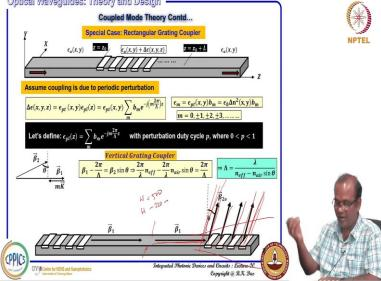
And this is nicely presented here you see this is your beta 1 incoming and beta 2 output. So, output if it is a guided mode if this grading is there it will be coupled. So, fraction all I will be coupling like this direction so what do you if you put a fiber along this angle this theta angle if a certain lambda is calculated then you will be getting theta if you bring it optical fiber and then light can be coupled into the fiber then.
