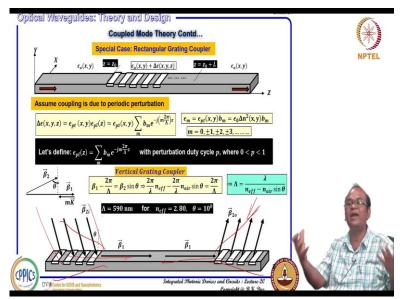
That since light can be coupled this direction. So, in the reverse direction light comes this direction 10 degree angle if it is incident on to the waveguide then light will be coupled to the guided mode also the reverse phase matching condition so that is counter propagating and co directional propagating situation like that. So, you can have in the input side also you can have a grating structure and you can bring your fiber.
