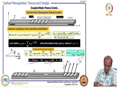
If a guided mode is having effective index of 2.80 we have calculated earlier for a effective index of guided mode that is in the order of 2.8 or something like that and if you want that coupled light into the air that should go in 10 degree then period requires 590 nanometer. So, you can define this period so that you can control light at 10 degree angle you can have completely 90 degree. So, for 90 degree what would be the theta value? Theta value will be 0.
