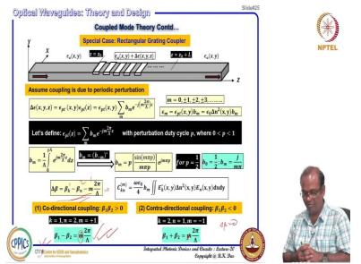
Now you will know that the another requirement is there couple mode equation is not enough but to get a meaningful coupling between 2 modes we have to have this propagation phase constant this longitudinal phase matching should happen for k = 1, n = 2, m = 1 we know beta 1 - beta 2 - m / 2 pi lambda that should be equal to 0. 1, 2 and m = 1 that should be equal to 0 that gives you beta 1 - beta 2 = m over 2pi lambda.
