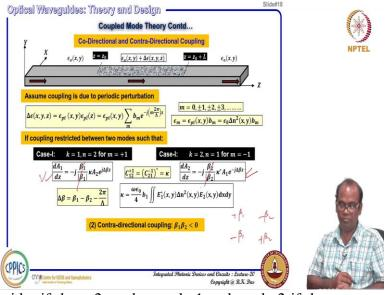
Now we will consider if these 2 modes mode 1 and mode 2 if they are counter propagating one is positive direction another is negative direction. So, when I can consider beta 1 positive and beta 2 negative if it is negative direction or beta 1 I can consider negative and beta 2 positive. So, in that case I can if I considered beta 1 is negative beta 2 positive then negative sign here negative, negative sign positive but here no sign change will be there.
