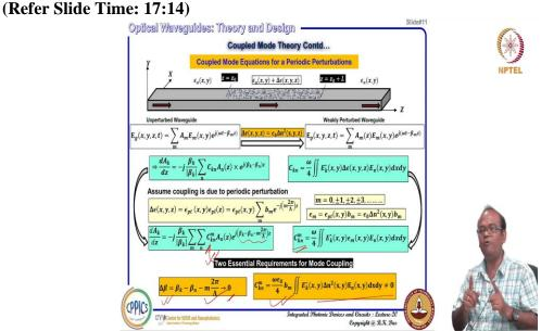
So, in this way we can conclude that 2 essential requirements for coupling between 2 modes. So, kth mode and nth mode what are those 2? One thing is that this longitudinal phase must be equal to 0 or close to 0 at least so that at least something will be building up if it is tends to 0 this periodicity phase mismatch periodicity will be long enough but you can get in the meantime some coupling.
