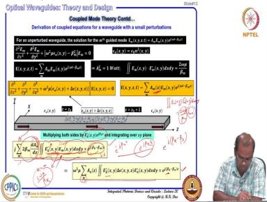
So, left hand side and right hand side I have written into 2 box, let us see here. So, first E k star x y E m x y dx dy and I have multiplied E to the power j beta k z, and originally it was e to the power - j beta m j z was there. So, if you multiply then you are getting e to the power j beta k - beta z and E k star I multiplied here E m this one and dx dy where you are integrating this one.
