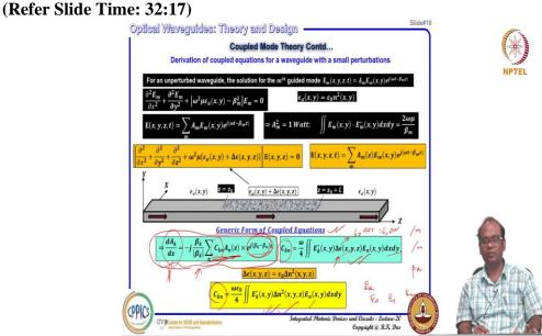
So, this is called actually generic form of coupled equation. So, this is the equation it is very, very important is the base of couple mode theory of course, it is a weekly guided coupled mode equation, why it is coupled mode, you see it is coupling kth mode to all other mode via these terms this is the sum so, you are for kth evolution, you see the contribution coming from all the modes and how that contribution coming because of the perturbation.
