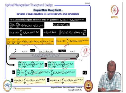
So, we can just now clean up that, this is del 2 E del x 2, del 2 E del y 2, del 2 E z 2 this has a 2 terms. So, what is next, next is you just insert all these 3 terms here, here, here, multiplied by E here, you just inserting in this equation. So, once you insert, then what you return back you get first term whatever you are getting that should be added with these should be added with this.
