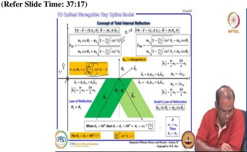
If I just do a little bit work on it, you see cos theta t I can write like this, because this one greater than 1 I have just taken j outside j = square root of minus 1. So, if this is j kt is imaginary I can just write this one for theta i greater than theta c that means, in complex form I can write, how to write?
