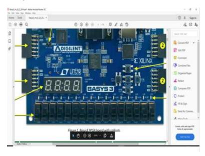
The other thing which I would like to point out here is the numbers which are written here, so for example this is the LED 0 and here E19 is written and for LED0 u16, so this is the u16 number is written LED 1 u19 is written. So, what is this u19, u16, et cetera, so this is our FPGA chip, on the FPGA chip there would be various pins, these pins numbers are written here that means there would be several general purpose pins these.
