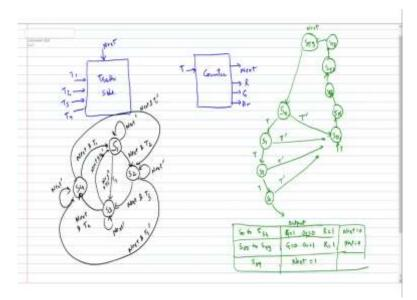
So, in that case, let us try to divide our state machines into two different ones. There are two state machines let us say this is first state machine, this state machine is taking input T1, T2, T3 and T4. This state machine is trying to decide that which particular side we are. So, which particular traffic side is working and what is the output to this, let us wait for a moment for that and the other state machine is a counter.
