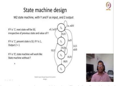
So, if that is given as a input, what would be the effect? So, first thing is that because first thing is that F is 1, so, that means I have reached 255 states. So, that means it is the end of the block. So, that means, whatever is my present state it does not matter. Whatever is my present
