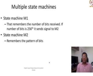
Now, let us look at let us try to say that this the first state machine, which is just counting how many bits has been received, let us call it M1 and M2 is the bits, which is remembering the pattern of the bits, how many bits has already matched. So, now what would be the interaction between these two state machines?
