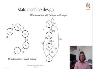
So, the M1 is straightforward that because it does not have any input and only F is the output so, what it can we can do is we can simply make it a state machine which is a counter S0 to S1 then S2 then S3 then S4 up to S255 and in all other cases output is going to be 0 but only when state is the final 255 states then the output is going to be 1. So, that means all the inputs has already received.
