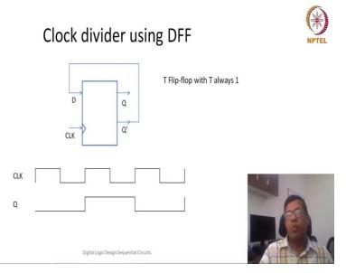
Now, let us look at the other application. So, can we design a clock divider using D flip flop. So, rather than looking at so this is my D flip flop so rather than looking at design, what I am trying to show you is the direct implementation Then we can analyze that how it is working. So, if this is the, this is my D flip flop, and I know that whenever clock, so whatever is, given the clock was the edge of the clock, this D would be transferred to Q.
