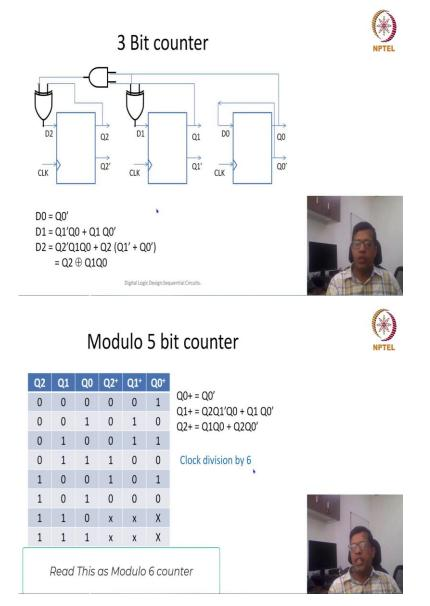
So, I can say that D0 would be equal to Q0 dash D1 is equal to Q 1 XOR Q0 and D2 I can simplify this equation as Q2 XOR Q1 Q0 and again implement this using these 3D flip flops where D0 is equal to Q0 dash and D1 is equal to Q1 and Q0 is XOR and D2 is equal to XOR of Q2 and AND of Q1 and Q0.
