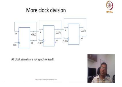
So, for that, I can repeat this circuit. So, because of this one circuit, my output is clock by 2. Now, if I give this clock by 2 as a input to next D flip flop. So, I connect this Q to next clock and then the output is going to be clock by 4. So similarly, I can connect it further I can further connect it and then I can say that this output will go as an input clock for the another D flip flop so then this output signal is going to be clocked by 8.
