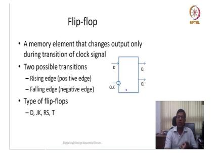
These storage elements memory elements, which can store the input at precise synchronization point or precise transition points are called flip flop. They are also called, so they will only change the output during the transition of clock period, they will not otherwise change their output. Now, output will change and we have seen that there are two transitions one is positive edge or rising edge.
