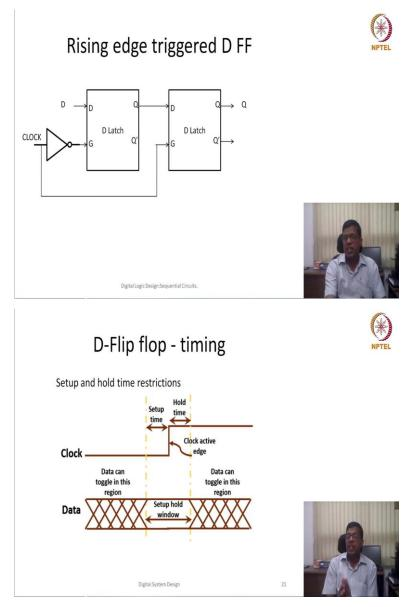
So, let us look at in this circuit whenever this circuit was, this clock was negative or clock was 0 that means this gated input was 1 so, that we whenever it was 1 at least sometime before that what should be, whatever should be the value of D, will go in the output of first latch. Similarly, because it was available at some time before the latch and whenever this particular gated input become 1, then only this can go and transfer to the Q.
