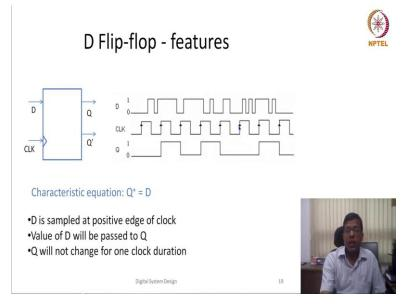
Now, a delay flip flop is represented by a characteristic equation that the next state is equal to D. Now, you see there is no control signal. So, at what time Q plus or next state would be
