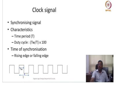
So, what is this precise time? For this, I will take a small detour. And I will try to explain one of the very important synchronization signal that is called clock. In most of the digital circuits, this clock signal or a clock wire is a very one of the very important signals because it synchronizes, what do we mean by synchronizes.
