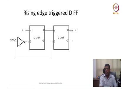
So, now how can we design how we can implement using our basic gates this kind of a D flip flop design can be done using 2 D latches. So, if we have 2 D latches one is one is gated with a with a clock signal which is inverted, the other which is which is gated with a clock signal, then we can design this rising edge triggered flip flop. So, what would happen because the clock is inverted.
