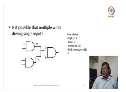
So let us take this example. Let us say I have two AND gates. These two AND gates, one of the AND gate has output Z1. Other has output Z2. Now both of these outputs are going to one input A. So what would happen in that case? We have to understand that these are all wires. This wire is connected to this wire. And when, let us say, consider that when there was only one, each input was received from one output.
