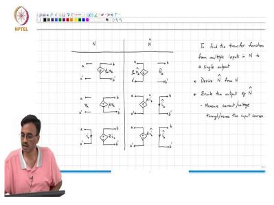
So therefore, in N if we had a voltage controlled current source. So, this is a, this is a prime this is b, this is b prime this is gm v a. Then in N hat we have a, a prime, b, b prime, v, v prime, this is g m. Now, this is a voltage controlled current source. So, I am not going to sit I mean here we did the derivation and found this you can do the same derivation for the other controlled sources. There I will give that as a part of the homework, so that you are convinced.
