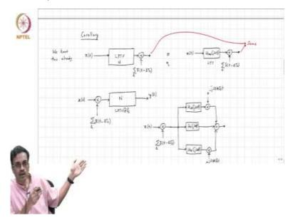
So, the next thing that I would like to talk about is a corollary of our principle that we have seen so far or I would send you all I would say. So, so far we have seen that if I have an input into an LPTV system and we sample the output at nTs. It does not matter whether it is nTs or nTs plus t naught. We know that we can always find an equivalent LTI system. We said that this is equivalent to have x of t driving an equivalent LTI filter, and if you sample the output.
