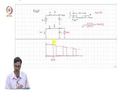
And we were considering an example, we will continue with that this afternoon. So, this is vi, this is R, this is c, this is v out, and this is phi. This is Ts, and this is d times Ts. And to find and let us say we are interested in v out of n times Ts. And what to do that, we basically understand that we can think of this as vi, pass through h equivalent of t and the output is sampled at nTs, so we will get n times Ts.
