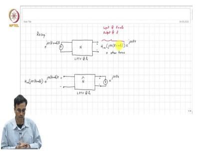
A quick recap of what we were doing in the last class. We saw the frequency reversal theorem and we were applying it to a practical case of chopped amplifiers. So, let us quickly recall what the frequency reversal theorem is and while, in this picture we show a current excitation and a voltage output, the same thing can be extended to other kinds of inputs and outputs. And one form of frequency reversal theorem is shown here.
