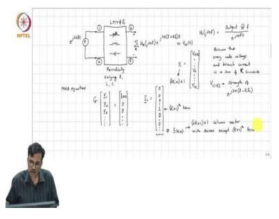
Again, to begin with we will restrict ourselves to networks with so this is LPTV at fs and again this is node 1, I will choose this to be node 0, this is node 2 and this is node 3, I will excite it with an input current which is e to the j 2 pi ft and I will measure the voltage at the output and the voltage as you know is not only consists of f but all components which are variable.
