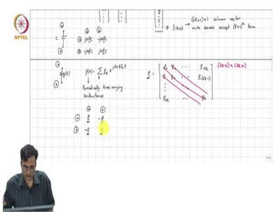
So, and what is G? G is again the sum of the MNA stamps of all the elements and what are the MNA stamp of a capacitor connected between nodes say a and b, a and b yeah, very good, so what will we do? Well, in the matrix you have this j 2 pi fc minus j 2 pi fc minus j 2 pi fc and j 2 pi fc.
