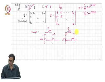
So, for example, let us say you had a switch in N which was controlled by some phi of t which did, so let us say this is t0, this is t equals ts. Now, what would the, so in N hat, you would have the same switch controlled by phi hat of t, so this is phi of t and phi hat would basically look like this so this is t equals 0, this is t equals ts. If you have multiple switches you basically do flip for everything.
