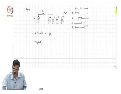
A quick recap of what we were doing yesterday, we were looking at what is called N-path filter example of which, so you have four identical capacitors and these are the clock waveforms and this is Ts, this is a 25 percent each one of these clocks this is phi 1, phi 2, phi 3 and phi 4, each one of these waveforms is a 25 percent intuitive cycle clock.
