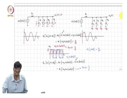
So, to do that let me copy this over, as usual we put in cos 2 pi; cos 4 pi fs times t and sin 4 pi fs times t this is Wi of t and this is Wq of t. And what are the voltages on this capacitor? Well the, if you have an input which is at twice the switching frequency then in one quarter of the clock period you basically have one half of the input cycle, then, so this is Ts, so this is cos omega t.
