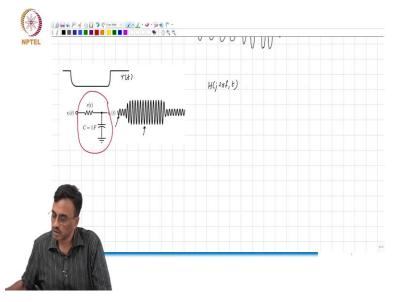
So, here is an example. So, this is r of t and when r goes down you expect the bandwidth to increase and therefore, the output should be expected to increase. It is not apparent here that the phase shift of this sinusoid with reference to the input is different from the phase shift of that sinusoid and to therefore, find H of j 2 pi f comma t, what should we do?
