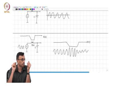
Let us now make this a linear time varying network. So, now what I am going to do is vary this resistance, say like this. So, the resistance is constant for a long time and I pulled t down, so this is R of t. So, what do you expect qualitatively to happen? The input is a sinusoid it is some frequency. What do you expect to see at the output?
