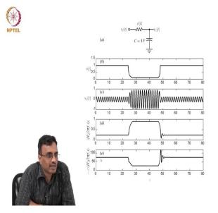
So, this is an example where, so r of t varies as you can see here and you can see that the envelope of the sine wave does indeed increase with and eventually once the r becomes small, you can see that the envelope actually increases and it turns out that in this case the, what do you call the bandwidth initially is 1 hertz and finally the bandwidth is if you look at it I thinks it is one eighth of a hertz so something like that.
