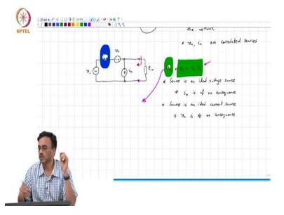
And so, a couple of observations. Let us say for example, that we are driving the network with some Rs, and then here is va and here is ia and this is the internals of the network. So, there is some Rn here that represents the input impedance of the network looking in. So, what comment can you make about the, what comment did we make about dividend voltage looking in here?
