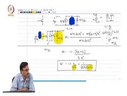
Now, let us do a simple common source amplifier whose incremental picture is shown here. And this is VI, this is Rs, and that is RL. So, what comment can we make? How do we, what is the noise factor? What do we do? First thing is to find the total output noise. So, what will be the total output noise, noise spectral density?
