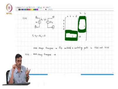
The next thing is basically the current-controlled, we have seen the voltage-control current source, the voltage-controlled voltage source, the current-controlled current source and the last man standing is the current-controlled voltage source, and how will this look like? So, you have a, again, we have 0 voltage source and this is 0 volts, this is ix and what are the, this is node c, and node d, and this is some z some impedance times ix. So, how many unknowns do we have now?
