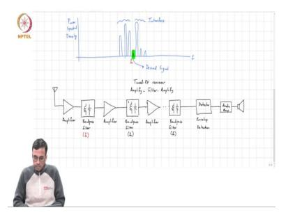
How does a modern phone do this? Well before we get to the modern phone; let us step back in time and see how radio receivers were built you know almost 100 years ago. So, the received signal which was received by an antenna would be very very small; and as you have just seen and to be able to figure out what received signal looks like. The electronics that follows the antenna must be able to see a sufficiently large signal. So, what is done or what was done was to have an amplifier up front.
