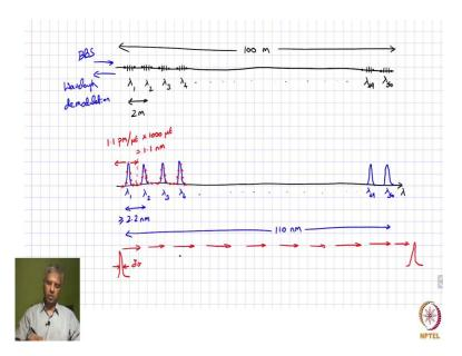
So, let us come back here and then try to capture all that information. So, for the bridge monitoring application delta lambda is equal to 110 nanometers. So, what does that mean as far as this filter function is concerned? You want to make sure that there is only one peak that is present within that 110 nanometers. So, going back to this picture again.
