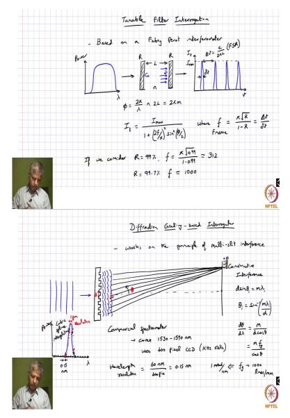
So, one example of that is this fiber Fabry Perot interferometer that is made by Micron Optics. Essentially, like we showed, two fibers whose ends are coated, and they could, depending upon the mirror coating, they could support wavelengths in this range. But the key thing that we want to look at is what is the free spectral range that you are interested in for your sensor system and what is the finesse you are interested at.
