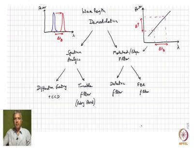
Now looking at wavelength demodulation techniques for fiber Bragg grating base sensors, and hope that we realized that one family of that is spectrum analysis and within that we were discussing this diffraction and CCD based interrogator.
