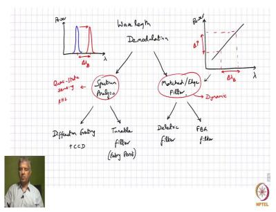
So, the spectrum analysis is typically for Quasi-Static Sensing. So, that is over kilo hertz, but it can handle really large number of sensors at a time. But if you want it to go to true dynamic sensing and if you do not have that many numbers of gratings to interrogate, because if you have only a few gratings, the cost that you incur in doing the spectrum analysis it is not something that you can justify very easily.
