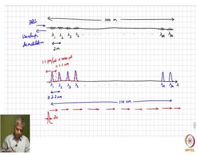
So, for example, if we consider the case that we had over here for bridge monitoring. So, we talked about requiring 110 nanometer spectral width. So, we need to be able to capture spectrum across this entire band, and how can you do that? Using a tunable filter, essentially, if this is the spectrum that is coming towards the receiver, you need to essentially have a tunable filter whose peak can be swept across all the spectrum.
