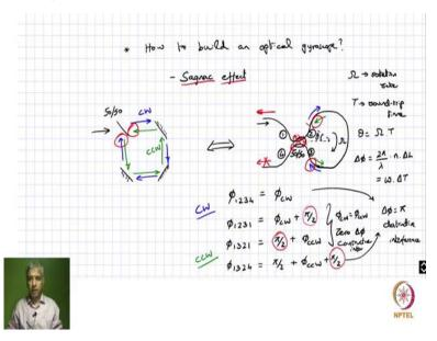
During our last lecture we were talking about fiber optic gyroscope and we were looking at the principle of behind the fiber optic gyroscope, which is, what we identified as a Sagnac effect, so essentially we are looking at phase changes between clockwise propagating waves and counterclockwise propagating waves and there, these are the counter clock wave, counterclockwise propagating waves.
