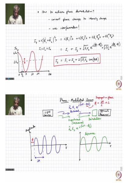
So, the question is, how to achieve phase demodulation? So let us look at that. Well, essentially, what do we mean by phase demodulation, it is such that whatever phase changes we wanted to detect, we are converting to intensity modulation. So, what we are trying to do is convert phase changes to intensity changes. So that is what we are trying to do. And what is a good way of doing it? Well, one of the common ways of doing it as far as optics is concerned, is actually use interferometers.
