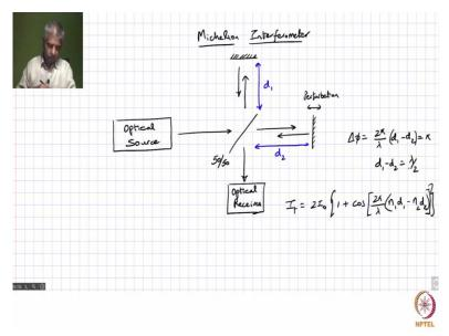
\* How to achieve phase demodulation? - convert phase changes to intensity changes - me interferometers!  $I_{F} = \langle |\bar{E}_{1} + \bar{E}_{2}|^{2} \rangle = \langle |E_{1}|^{2} \rangle + \langle |E_{3}|^{2} \rangle + \langle E_{1} + \langle E_{1} + \bar{E}_{2} \rangle$   $I_{1} = I_{0} = I_{1} + I_{2} + \int I_{1}I_{2} e^{j(\theta_{1} - \theta_{2})} + \int I_{1}I_{2} e^{j(\theta_{2} - \theta_{1})}$  $I_{t} = I_{1} + I_{2} + 2 \int I_{1} I_{2} \cos(\Delta \phi)$ 38 27 40
