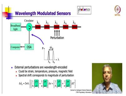
So, to understand this, let us consider this sort of schematic you have broadband light, which is going through this device called a circulator. Circulator essentially directs light from port 1 to port 2, but any light coming from port 2 would not go back to port 1, instead it will go to
