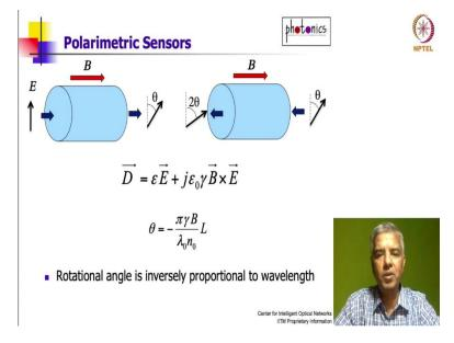
So, let us go into what are called polarimetric sensors. To explain this, I will have to explain something that is called the Faraday Effect. So, what is the Faraday Effect? Well, you can come in with light with a particular polarization linear polarization, let us say and it can go through this material which has, what is called a very relatively large magneto gyration coefficient. So, what does that mean?
