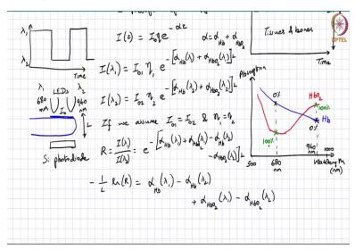
Let me see if we can go down a little bit, you can rearrange those terms and then you can basically get an expression in terms of the measured quantity. So, what is measured, is actually the ratio. So, from the measurement you need to infer the oxygen saturation. So, you can rearrange it as so, this will become minus 1 over L log of R is is going to be given by just alpha Hb of lambda 1 minus alpha Hb at lambda 2 plus alpha HbO2 at lambda 1 minus alpha HbO2 at lambda 2.
