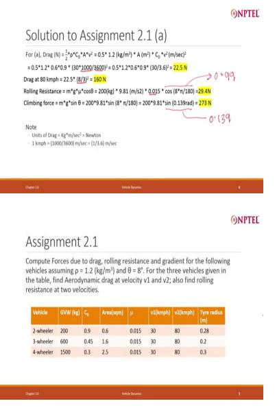
For 2.1 A, the drag what is a drag coefficient? I have mentioned it was half rho CD A into v square, half is 0.5 rho is always 1.2 kg per meter cube area into CD into V square and therefore I have put here 0.5 into 1.2 and area for the first vehicle is 0.6 square meter. So I am actually
