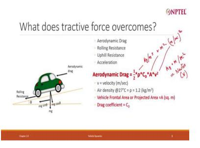
A vehicle, see this vehicle here, this vehicle actually undergoes one of the forces that it undergoes. There is aerodynamic drag, the vehicle is moving in this direction, there is aerodynamic drag which is trying to push the vehicle back, this is called aerodynamic drag.
