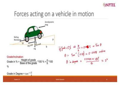
Before I proceed, I want to talk about this theta, how is this gradient defined? Suppose the gradient is defined in terms of 5 percent, suppose if gradient is 5 percent, it is 5 percent that means p by b is 5 that is what it means. So 5 percent implies p by b is equal to 0.005, sorry yes 0.05 I made a mistake, 0.05. If the p by b is 0.05 what is a gradient? This is tan theta is p by b, so this tangent of theta.
