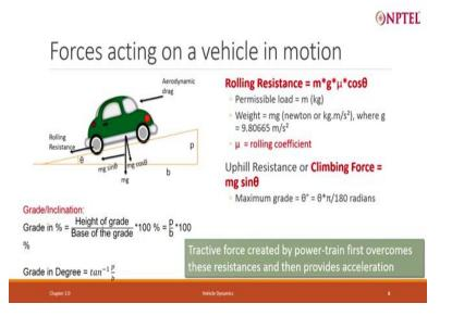
So basically I have sort of say you will often get a slope vehicle has to travel up a slope and when it travels up a slope you will have to define theta, theta can be defined in percentage, very often it is gradient in percentage; 5 degree, 8 degree, 10 degree, (sorry) 10 percent, 5 percent, 8 percent.
