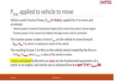
So now I am ready to say what is the total traction force. Vehicle needs a traction power applied for it to move and accelerate. So traction power has to be minimum as sum of the 3 powers; the aerodynamic resistance, rolling resistance and climbing force if there is any climb that will just be enough to keep it moving and if I want to accelerate I will need more power.
