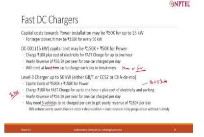
What about fast DC chargers? Now I am moving away from AC charger and we are coming to DC charger. So, if I take a 15 kilowatt DC charger. Power installation itself may cost you 50 kilowatt 50000 rupees because you are doing 15 kilowatt again you will require a special line. Electricity board will say oh to give you a line I will cost take 50000 rupees. For larger power of 50 kilowatt they may charge 1.5 lakh.
