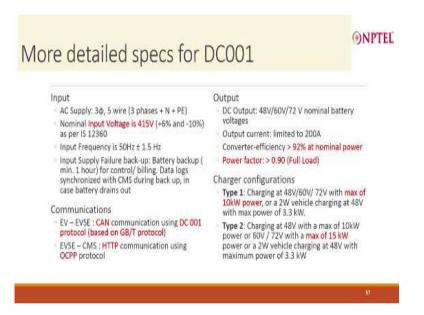
So more on that the input side supply is actually the same that are there for AC charger we use AC 3-phase and all the conditions that we apply on it for the threshold tolerances etcetera are followed as per IS standards that we have and extra things that we have is the battery backup for billing purposes like we have it in AC charger and OCPP is what we follow from EV to EVSE.
