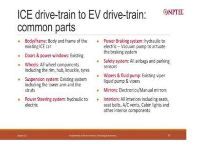
So, start with some of the parts which are common. For example, body and frame. Well, body and frame is required for petrol vehicle, it is required for a electric vehicle. Now, there are changes that you can make.
