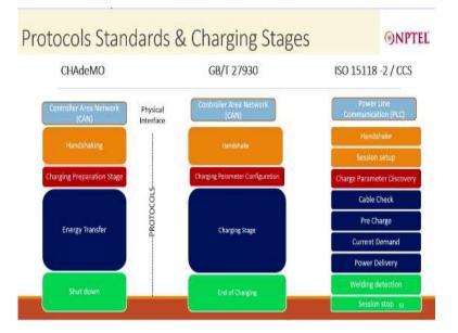
Protocols that we have discussed so far for DC standard that is Chademo, GB by T ISO-15118 which is actually CCS standard. At the protocol level the difference is between their physical media and their application layers that are divided into. As we are not covering every standard picked up into detail we just are laying out here the basic differences that are there. So if we talk about Chademo and GB by T both are the physical level use CAN interface.
