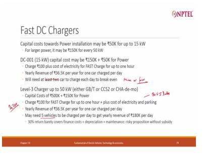
What about fast DC chargers. Now moving away from AC chargers and we are coming to DC charger. So, if I take a 15 kilowatt DC charger, power installation itself may cost you 50 kilowatt, 50,000 rupees, because you are doing 15 kilowatts, again you will require a special line electricity board will say, oh to give you a line I will cost take 50,000 rupees for larger power of 50 kilowatt they will charger 1 and a half lakh crore lakhs.
