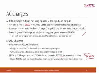
Start with the AC001, single output chargers 15 ampere plug point and you are trying to charge a two wheeler or maybe a three wheeler or even a small four wheelers about, let us say three four hours, slow charger. Normally a 230 volt input and output will be what the vehicle needs. A simple outlet like this, what does the outlet consist of, outlet has a essentially AC plug with all the protection.
