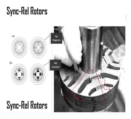
This an area of active research and so as I told you this will be the kind of rotor that have no magnets at all and these are rotor where there is a little bit of weak magnets. That is called the PM assisted magnet and this is how a PM assisted magnet would be assemble those little magnets are going into to the slots. What you can see here is that is the d axis and as you can see in the d axis there are large air pockets and magnets are as good as air. Or as bad as air in terms of reluctance.
