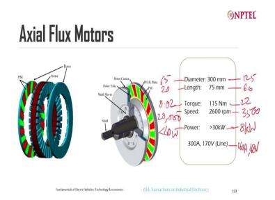
And another area which is interesting is what is called axial flux motors. Here the magnetic lines are parallel to the axis of rotation which is very funny. This is a rotor and this a rotor both the rotors they are like slices with magnetic poles facing each other and in between is sandwich the stator with the windings. And at the core of every winding in the conventional architecture we saw that the core is the teeth of this stator.
