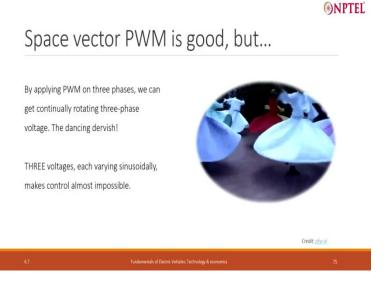
So the challenge is that while the motor needs AC, for us to be able to control the motor we need to look at everything from the d-q reference frame, where all the entities are DC. And so, while we apply PWM on the three phases to generate the AC, and the actual picture of the motor is that
