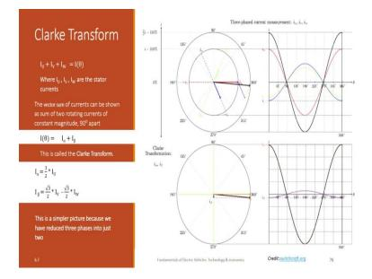
So how do you convert from AC to DC? We do it in two steps. The first step is called the Clarke Transform. We have already seen that when there are three oscillating currents in the three phases, they are 120 degrees apart from each other.
