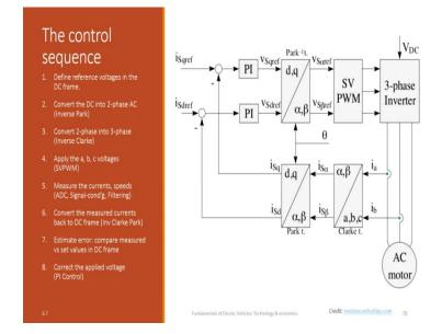
So having understood this, we can now understand how the whole control sequence works in the controller. Essentially, the first thing that we do is I want the motor to deliver certain torque, which means it must take a certain current and it must be running at a certain speed, which means a certain pair of Vd and Vq voltages have to be applied. This is what the controller decides.
