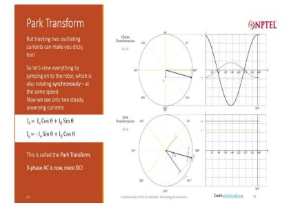
And we take advantage of this knowledge to do what is called the Park Transform because even with two phases if I were to go on looking at them and try to see where is it compared to where I want it to be and try to adjust and correct the error, it is very confusing, we cannot do it.
