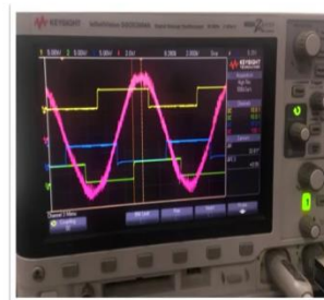
Shape of back-EMF measured on an oscilloscope
