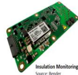
Insulation Monitoring Device. Source: Bender
