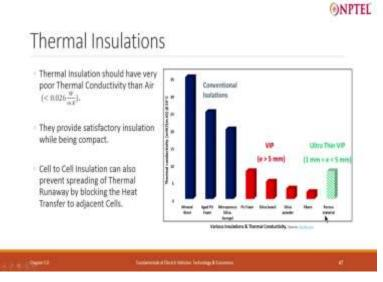
Now thermal insulation; where we require thermal insulation is order casing so that that my environmental conditions should not impact my battery much. If I have a passive thermal management system, I do not want to get it disturbed by environmental condition. Also, we
