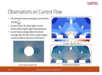
This map shows current flow, how the current is flowing. It is not uniform exactly. The current density the 4.35 ampere per mm square. So, you need to look upon how the current is flowing, it should be uniform basically. So, wherever there is a hole, because of that the
