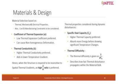
Coefficient of thermal expansion, we want it to be minimise otherwise, what will happen, we may develop thermal stresses. Thermal conductivity, mostly we want higher thermal conductivity so that heat can be transferred quickly. In exceptional cases, we do not want outside heat or environmental heat to be penetrated inside. In that case, we use materials which thermal conductivity is very low.
